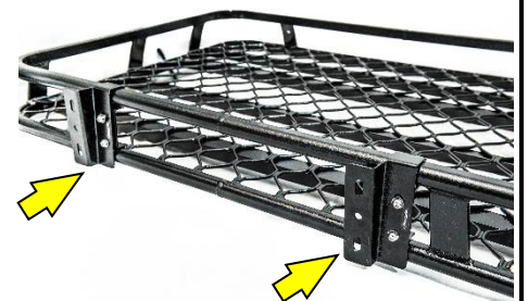
Fit second TLRAM Mounting Brackets to Side Rail, then tighten firmly. Fit Awning to the TLRAM Brackets, then tighten firmly.
