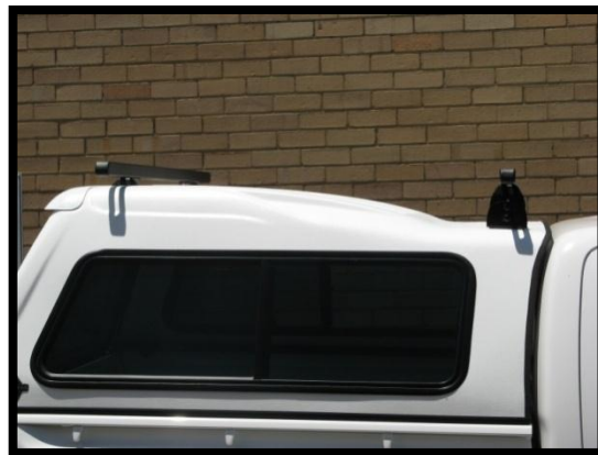
Rear and Front INTERNAL CANOPY BARS fitted to Single step- down canopy on Toyota Hilux Dual Cab Ute.
