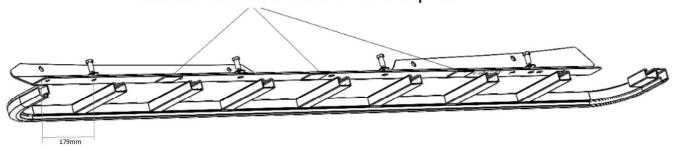
E. With the TLRAL22/FT/OE Roof Rack upside down, position the flat surface of the Tough Bars on the underside of the Roof Rack as shown above.
